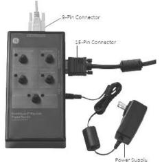
Don't fumble with connections or risk losing cables or parts ever again. The PSCGTUTK20 EntelliGuard Test Kit from Parts Super Center bundles GE's GTUTK20 Test Kit into a handy package that includes everything you will need in one place for field-testing EntelliGuard TU Trip Units.
